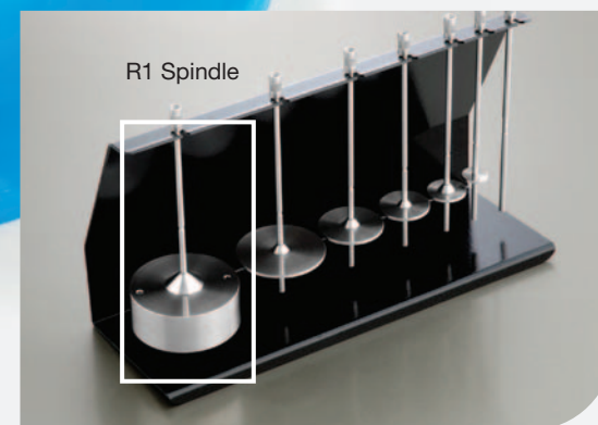
Standard spindles for R and H models. * The R1 spindle is supplied as an accessory
