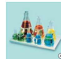
Basic tray with spring clamps
