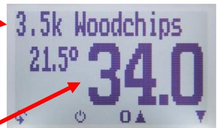
12. If the measure value is blinking, the valid measuring range is exceeded (limits see list on page 5). In this case the accuracy will be decreasing. If you are measuring wood chips, select the next higher weight class and refill wood chips to reach the higher filling weight.
