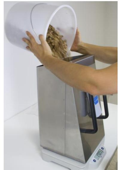
9. Remove material till the next lower weight range is reached. If only a little missing (e.g. 0,10kg) to the next higher level, it should be filled up to that stage. The actual weight is shown on the scale.
