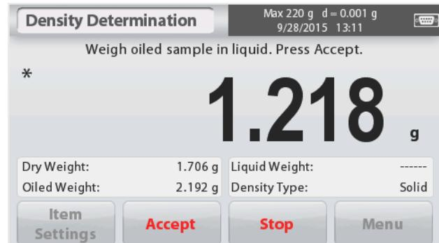
Once the necessary weights have been determined, the density of the sample is displayed in  $\text{g/cm}^3$  (along with the weight in air, un-oiled and oiled, and weight in water) on the Application screen
