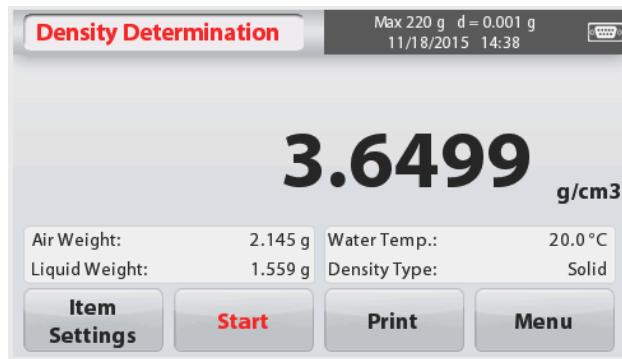
Press **Start** to reset all the weight values and restart the process.
