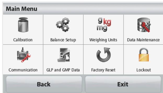
When the Security Switch is in locked position, the Calibration and Lockout menus will be hidden.
