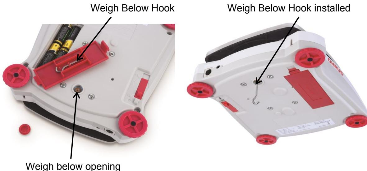
The balance can be supported using lab jacks or any other convenient method. Ensure the balance is level and secure and that the transportation lock has been released. Power on the Balance, then use a string or wire to attach items to be weighed.
