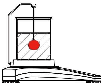
Once the necessary weights have been determined, the density of the sample is displayed in  $\text{g/cm}^3$  (along with the weight in air, weight in water) on the Application screen.
