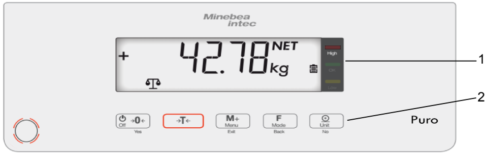
Front Control Panel with LCD Display.
