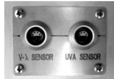
Figure 13: Lemo sockets to connect the light sensors
