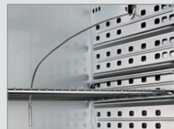
PT 100 sensor For accurate temperature measurement within the sample material
