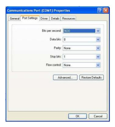
Make sure that RS 232 communication setting at the recorder and PC are equal.
