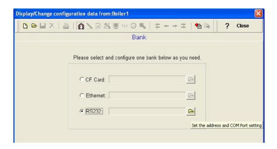
8. Set communication parameters for RS 232 communication at PC.
