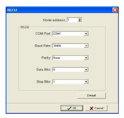
9. Click on OK after setting all above details. By default Node address is 1. If any change is there for the node address, then it should be set at recorder manually then enter the same node address in the above configuration.
