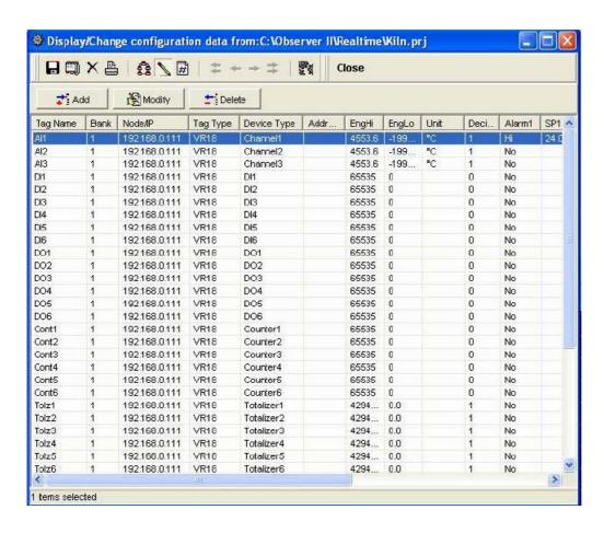
Double click on channel in the above spreadsheet to show the following Modify tag data with email configuration. If auto-update option is selected in modify tag data as shown in following screen, then all the settings done at the channel for events will appear here. If it is not selected, then user can configure manually for different set points in order to generating alarm emails.
