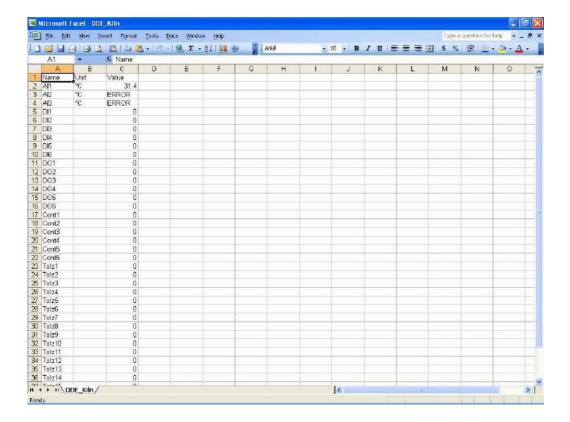
If any "Error" test appears in any cell of Excel, possible reasons is no data available at selected tag. Check the data availability at the recorder and Observer software for a particular tag.
