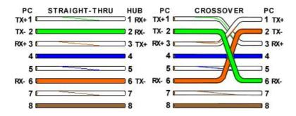
6. Connect proper UTP Ethernet cable as per the requirements and observe the communication status between the Recorder and PC/LAN HUB at the LED's dedicated for the purpose near female RJ 45 connectors.
