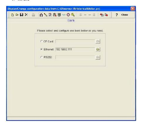
512 MB CF card shall be supplied along with the recorder. Standard Ethernet port (RJ 45 female) shall be available at the recorder. RS 232/ RS485 shall be supplied as additional options.
