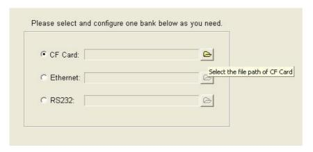
7. Click on to set CF path to receive the configuration data available in CF card.
