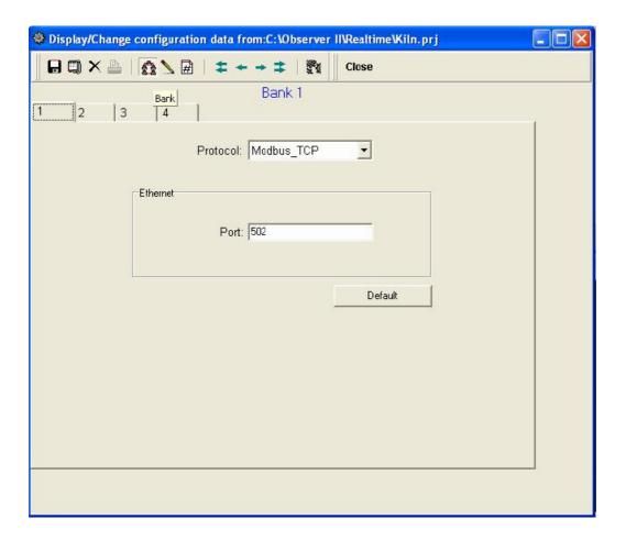
For Ethernet, Recorder uses port no. 502 for communicating with Observer. If you change the port number in Observer, you cannot establish communication between Observer and Recorder. Port no: 502 is used to establish communication between recorder and Observer software to exchange data on Ethernet over Modbus\_TCP protocol.
