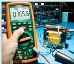
Measure the insulation resistance of transformer windings
