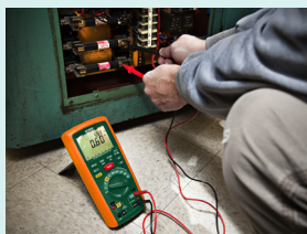
Checking voltage on a lathe
