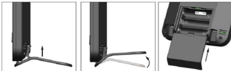
The WTH600 can be placed on a desktop or can be wall mounted for easy viewing.
