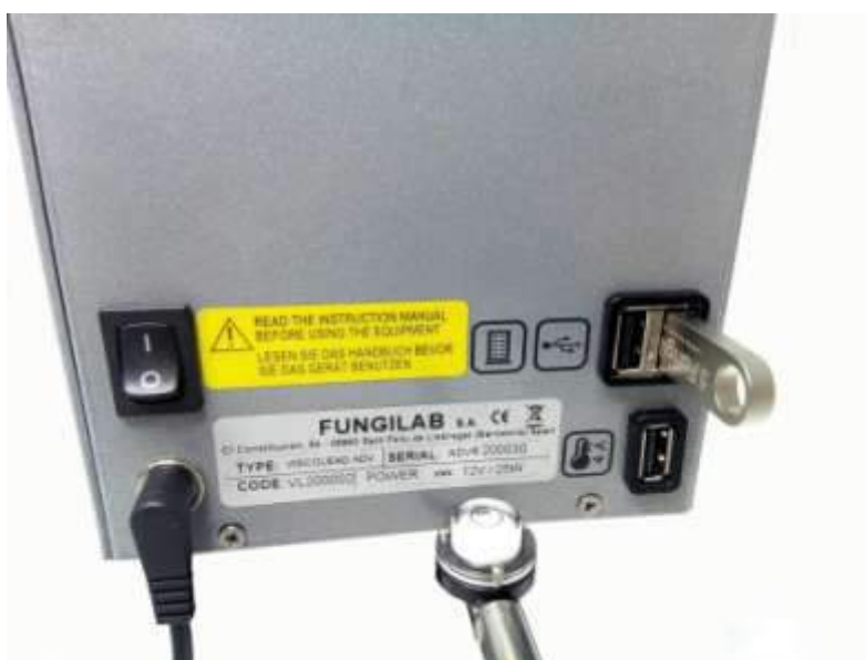
Fig. 7 USB-memory stick connection
