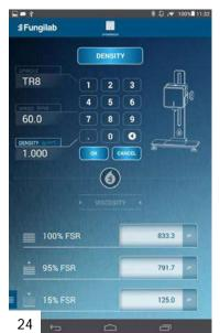
Press the density button to open the number pad [24].
