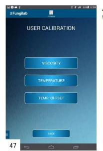
Allows the calibration of three parameters: viscosity, temperature and temperature offset [47].
