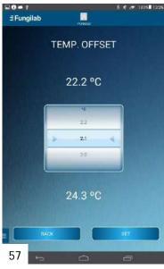
The temperature offset calibration screen displays a list with temperature deviations that the user can choose from. After selecting the desired value, press SET to complete the adjustment. The device will then be ready for testing.
