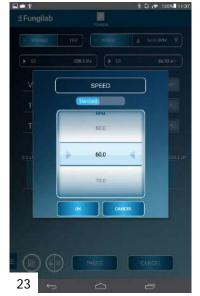
Select the desired speed by scrolling through the speed selection list. Confirm the speed setting by pressing OK [23].
