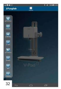
Users can create a customized test by selecting the PROGRAMS icon from the slide-out menu bar located along the left side of the screen.
