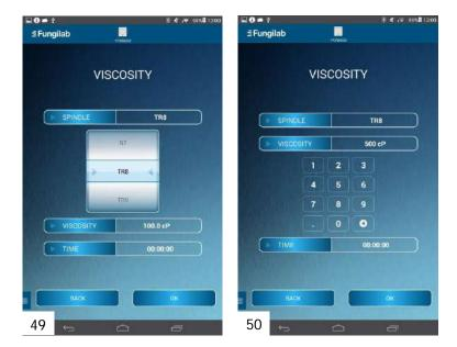
**Spindle Selection**: This is the unique spindle that will be calibrated, while the others will maintain the factory calibration.
