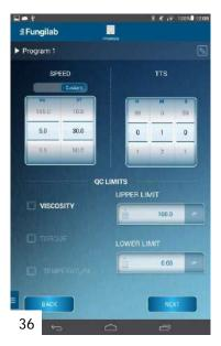
If RAMP is selected, the user must define the start and final speed [36]. The time can be increased but the minimum time value cannot be decreased. To select the Custom Speed function, a minimum of two speeds is required.
