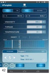
Selecting RUN will initiate the experiment. A screen will display program details, such as: spindle selection, speed, TTS and/or TTT, etc. [41].
