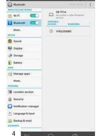
After selecting a product, the user will be prompted to pair the tablet to the device. To pair the devices for the first time, press the "+" icon on the screen [3]. This will direct you to the Bluetooth settings menu [4].
