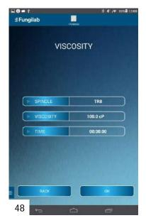
The viscosity calibration screen will display three parameters: spindle selection, viscosity value, and delay time [48]. By clicking on each field, the user can input new values [49][50].
