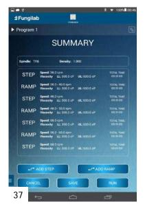
At any time, users can cancel the test, erase all customized configurations/settings and return to the initial program screen.
