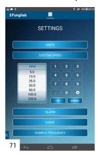
In the CUSTOM SPEED menu, users can add and customize speed settings for future testing [71]. To delete a custom speed, long-click the desired speed and the speed will be deleted automatically. The speeds will also be reorganized automatically.
