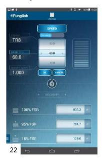
Press the speed button to open the Speed Selection list [22]. Above the selection list is a switch button to choose between Standard Speed and Custom Speed.
