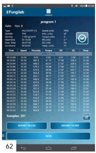
Users can access all recorded experiments in the DATA STORAGE menu located in the slide-out menu bar. The data storage screen will display a list of all previously saved tests [61]. Each experiment is labeled with a test name and the time and date the test was performed. Users can click on each experiment to view the results on a comprehensive data sheet. The results can also be edited and then exported in a PDF or CSV format.
