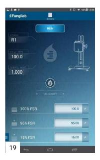
The MEASUREMENT CONFIGURATION screen displays several parameters that can be modified to suit the user's testing needs: spindle selection, speed and density [19]. The MEASUREMENT screen also displays the Full Scale Range values (see Section 6.4 for more information).
