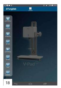
For quick-start measurements, select the first icon labeled MEASUREMENT from the slide-out menu bar at the bottom of the screen.
