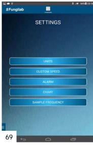
By selecting the SETTINGS icon on the slide-out menu bar, users can change the measuring units, custom speed values, activate the QC Limits alarm, customize each graph axis and input the desired sample frequency [69].
