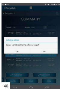
By selecting multiple STEP configurations, users can delete them simultaneously with just one click. [39].
