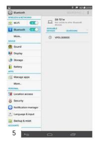
Once the search is complete, select the desired device from the list (the device will be labeled with the viscometer's serial number, ex. VPDX######). To proceed, the user must verify that the device's serial number on screen corresponds to the serial number on the back of the equipment's head [5].
