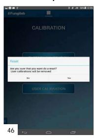
Completely resets the device, erases all saved data and reverts back to the original factory settings. All previously completed user calibrations will be lost [46].
