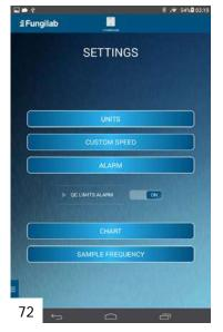
In the ALARM menus, users can activate the QC Limits alarm. The audible alarm will warn the user when the measurement is outside of the QC Limits. [72].
