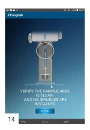
3. The user will be asked to verify that the sample area is clear and that no spindles are installed. Press ENTER to proceed [14].
