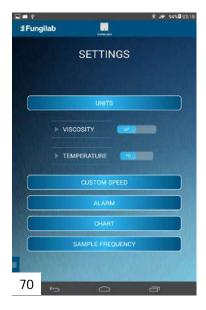
Viscosity units can be changed from millipascals per second (mPa·s) to centipoise (cP); Temperature units can be changed from Celsius to Fahrenheit [70].
