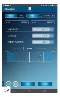
Users can set limits for the following three parameters: torque, viscosity and temperature [58]. Simply click each field to open the keyboard and input the desired values. Once the limits are inputted correctly, the user must check off the checkbox of the corresponding field.
