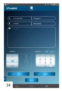
After clicking on the NEW button, the initial configuration screen will display three fields: program name, location and comments. These are optional and are completed at the discretion of the user [34].
