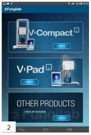
To begin testing, press the ENTER button located on the PRODUCTS display window [1]. Then, select the desired instrument from the PRODUCTS menu; you will then be prompted to pair the tablet to the equipment [2].
