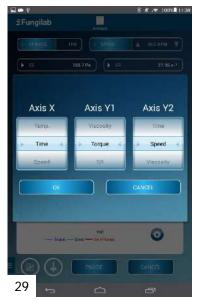
On the graphic display, a settings button on the bottom right corner of the graph will open a display window that allows the user to change the axis configuration. Once the graph has been configured, press OK to return to the graph display or press CANCEL if no changes are necessary [29].
