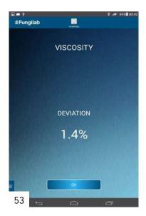
Note: After these steps, the APP will show a deviation of the quality of the calibration. The permissible deviation should be less than 1.5% and as low as possible so that the inputted viscosity in within the calibration matches the real viscosity of the fluid [53].
