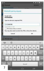
After selecting the desired device, a "Bluetooth Pairing Request" will appear [6]. This window will prompt the user to input the required PIN to continue [7]. Type in the 10-digit password that comes with your Fungilab product (this password is unique for each device). Press OK.
