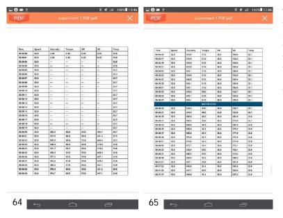
The exported PDF will also contain the same comprehensive data sheet found in the APP. The chart will include: time, speed, viscosity, torque, shear rate, shear stress and temperature values [64]. Any rotation interruptions during the test will also be shown [65].
