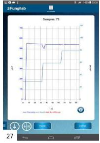
Users have the option of viewing data on a dual view display (graph and numerical values) [26] or a full-screen graph [27].
