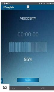
After pressing OK, an image will appear prompting the user to install the desired spindle and adjust the head to the correct vertical position (as denoted by the mark on the spindle) [51]. Press ENTER to initiate the calibration process. After the viscosity calibration is complete, the device will be ready to work.
