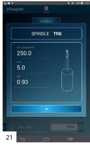
Click on the spindle button to open the Spindle Selection list. Scroll through the list to choose the appropriate spindle for the test [20].
