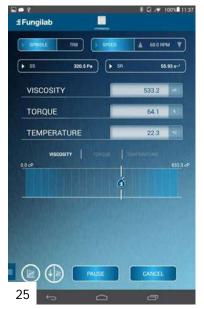
Once all the parameters are set, press RUN to proceed to the measuring screen. At the top of the screen is a quick summary of the selected parameters, as well as shear stress (SS) and shear rate (SR) values (if the selected spindle allows it) [25].
