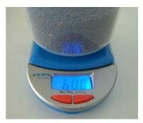
7. Fill up the measuring device with the sample material. The filling needs to be done slowly and constantly to ensure reproducible results. There must not be used a funnel or anything similar for filling.
