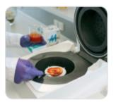
For samples with a high moisture content, microwave drying is the fastest and most effective thermogravimetric method for moisture analysis. Developed for analyzing moisture content ranging from approx. 8% to 100%, the LMA200PM performs moisture analysis in a fraction of the time it takes for other methods.
